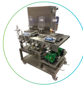
Virus inactivation system
