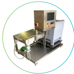
Continuous clarification system after USP
